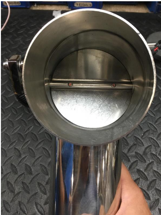
**Proper valve disc fitment **Valve disc conforms to the inner diameter of the tube
