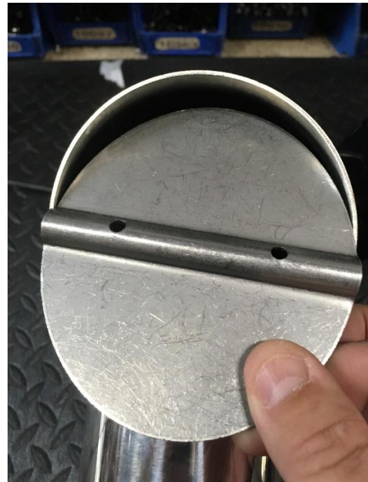
**Improper valve disc fitment **Valve disc does not fit into tube
