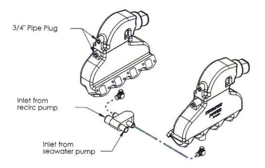
Water flow diagram for Thumper Power big block manifold (old style thermostat housing)
